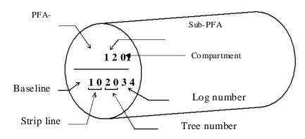
Note: This log harvested from PFA 1, sub PFA 2, compartment 01, base line 1, strip number 02, tree number 03 and log number 4.
