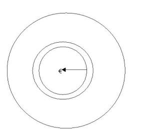
Centre: use to overlay the selected tree to be cut Circle 1: Radius with 25 meter used to measure the distance between two trees Circle 2: Radius with 30 meter used to measure the distance between two trees Circle 3: Radius with 56,4 meters used to count the mater tree per hectar
