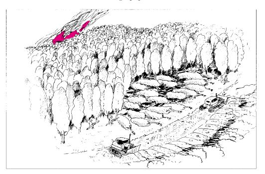
Bulldozers, fireline ploughs, and other heavy duty earth-moving equipment are extremely effective tools for building firelines, particularly in heavy fuels and brush. They must be followed by hand tools to finish the line, to burn-out where necessary, to hold the fire within the line, and to combat spill-overs and spot fires.
